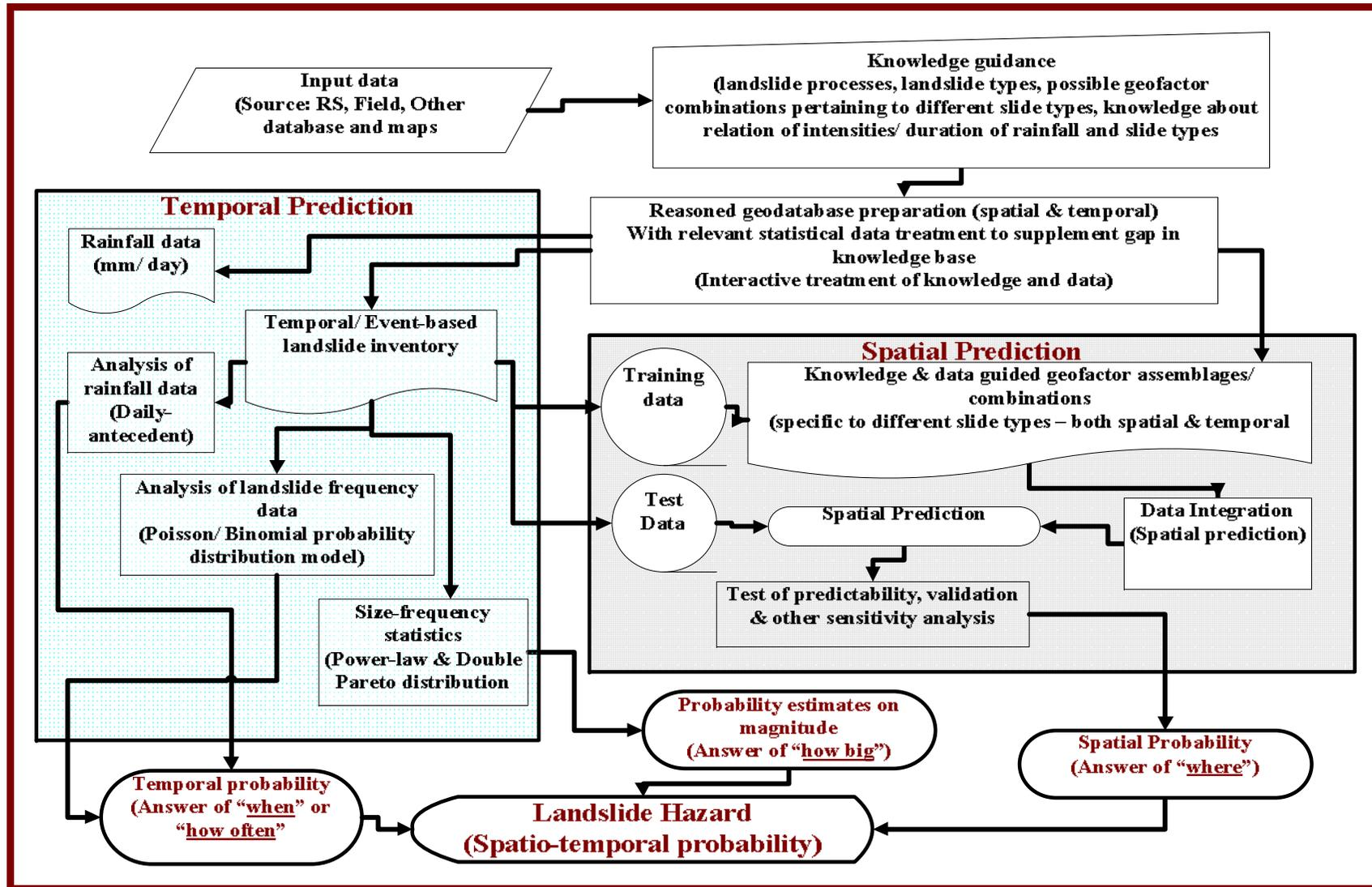
Figure - 1 = A general flow diagram of the knowledge-guided spatio-temporal prediction methods
